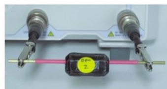
The unique signature of each ferrite is plotted from 0.1 to 450 MHz
