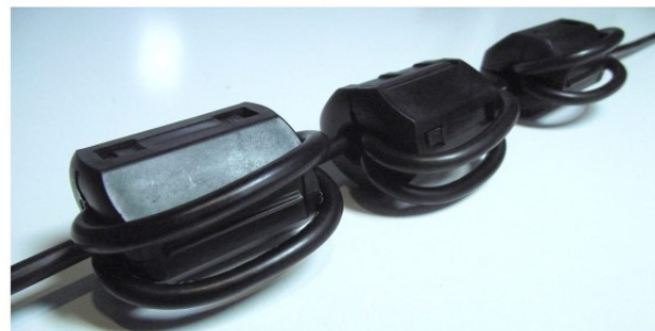
A run of RG58 coax on its way to a transceiver, via 3 large clamps, with 3 turns per clamp
